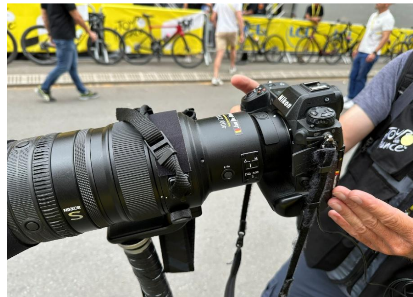
Photo reporter still camera equipped with a 5G modem to upload photos wirelessly from the finish line to the clouds of the press agencies
