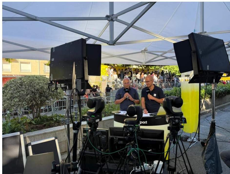
Test of 5G Live Studio operated in Remote Production from the Broadcaster's office
