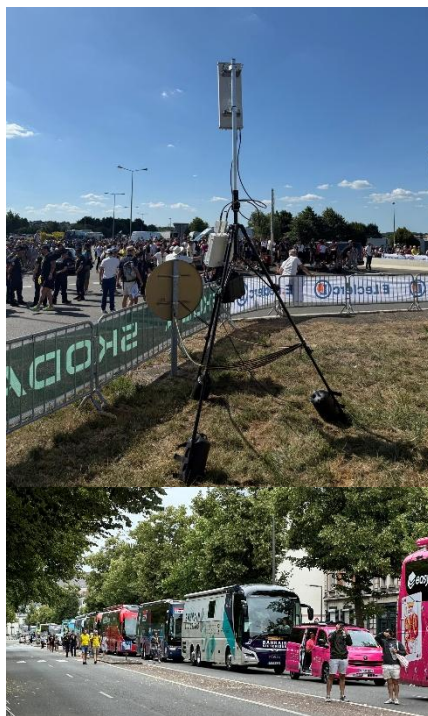
PRIVATE 5G NETWORK installed on tripod to cover the Team Bus area
