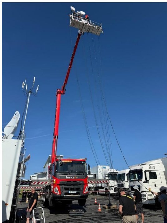
PRIVATE 5G NETWORK installed on crane
