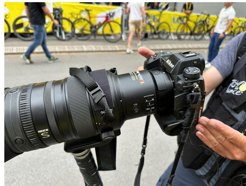
Photo reporter still camera equipped with a 5G modem to upload photos wirelessly from the finish line to the clouds of the press agencies
